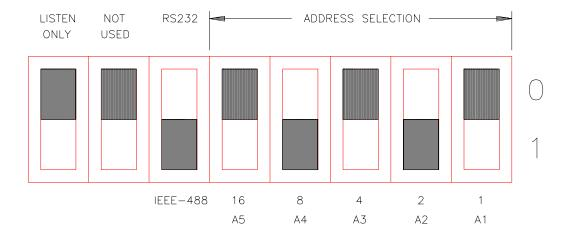
Figure 13-1: GPIB Address Selection Switch
